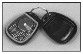
Notice: When replacing the battery, use care not to touch any of the circuitry. Static from your body transferred to these surfaces may damage the transmitter.
